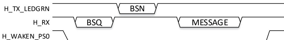
Figure 10: UART-SHTP Sending a message to the FSP200
